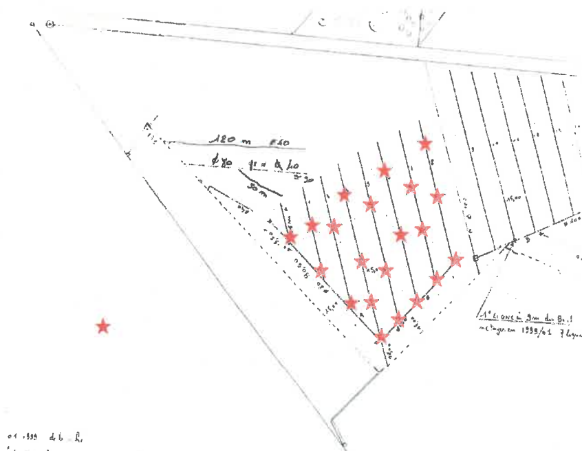
Figure 2. Bouchage des drains souterrains
